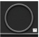
RFID antena fabricated on undoped ABS
